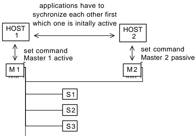
Once the DEVICES are started, the active Master 1 requests cyclically the assigned slaves and the passive Master 2 polls the Master 1 station, if it is still present. The APP 2 of the passive Master has to poll the COM bit in the cell bHostFlags, which reflects the current status of the M 1 station.
