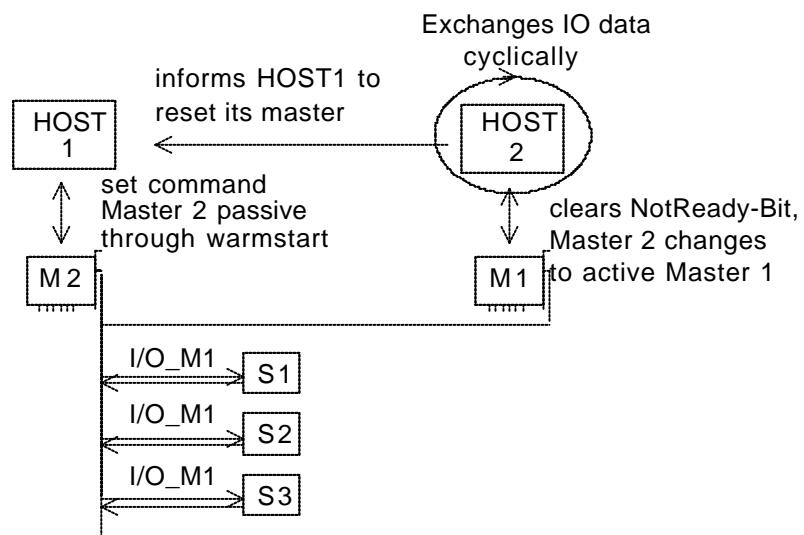
Another scenario that can happen is that the HOST application of the active Master 1 dies. To prevent that the active Master 1 then is still running without having valid process data and no valid HOST application running above him, the HOST application should support the Watchdog-Trigger mechanism, which is explained in the Toolkit General Definitions manual.
