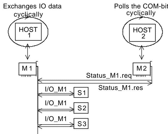
If the active Master 1 now dies, the status requests of the passive master 2 are not confirmed by the Master 1 any longer and the HOST in the Master 2 sees the COM bit in the cell `bHostFlags` gone. The IO exchange to the slave devices is stopped in that moment the master dies, but the watchdog functionality keeps them alive for a short time.( this time depends on the settings in the bus parameter of the master 1).
